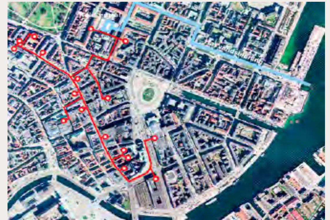
Figure 4.3 District cooling in central Copenhagen around Kongens Nytorv
